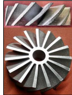
Figure 10. Abrasive-waterjet-machined aluminum blisk with the use of the A-Jet
